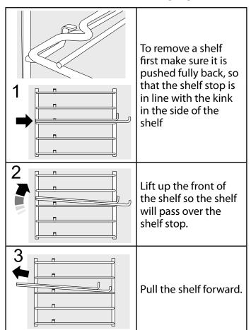
To refit the shelf, hold it so it is slightly up at the front and rest the back of the shelf on the side wires. Push the shelf to the back of the oven and then lower the front so that it is resting on the side wires.
